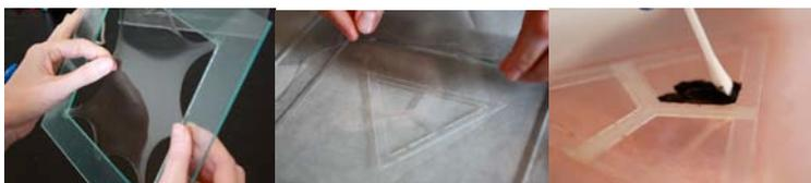
2 Elastomer pre-stretching, frame lamination, conductive coating
