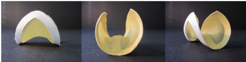
3 Minimum energy structure made from pre-stretched jersey fabric
